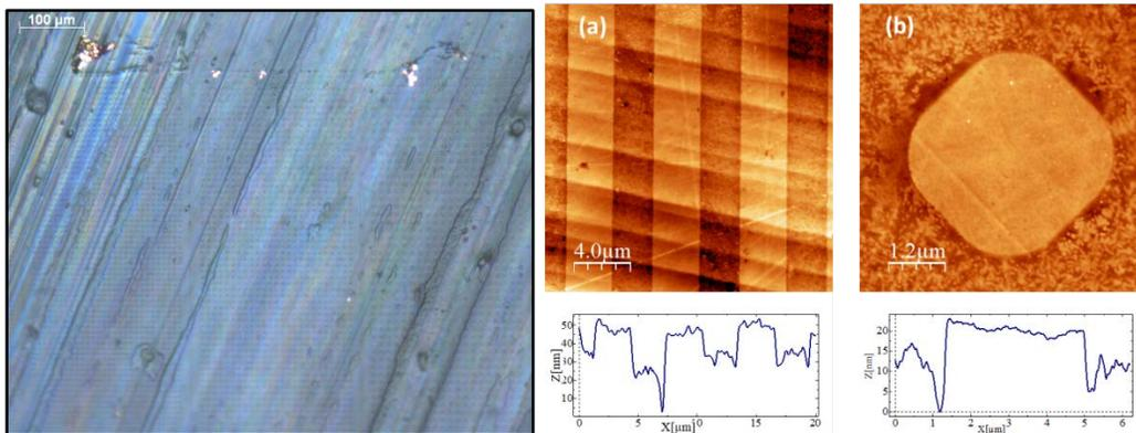
Figure 3: Transfer microstructures replicated on plastic by injection molding
