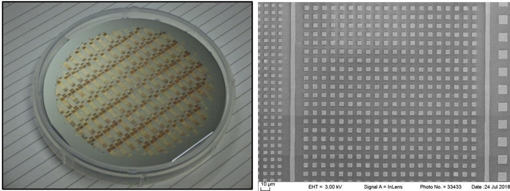
Figure 2: 4" wafer scale transfer of photolithographed structures
